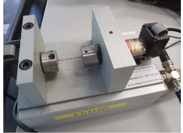
Fig. 7: Photo of the rotational two-mass-spring-damper (MSD) experimental setup used for measurements. The sampling rate of the encoders is set to 1048 Hz.
