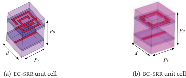
Fig. 7. Unit cell of NRI resonant metamaterials constituted of BC-SRR and EC-SRR and metallic lines. These inclusions are printed on the dielectric teflon substrates ( \epsilon = 2.2 , \tan \delta = 9 \times 10^{-4} ). The periodicities P_H=4.5 mm, P_T=3.3 mm, and d=3.3 mm.
