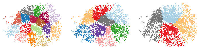
Fig. 9: Association of antenna sites to level- \ell nodes in the large metropolis scenario. The plots refer to \ell = 8 (16 nodes, left), \ell = 9 (8 nodes, middle) and \ell = 10 (4 nodes, right).
