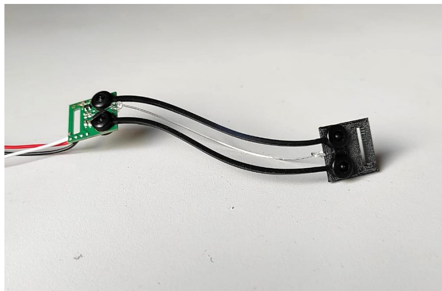
Figure 2. The electroresistive band used in the experimental test.
