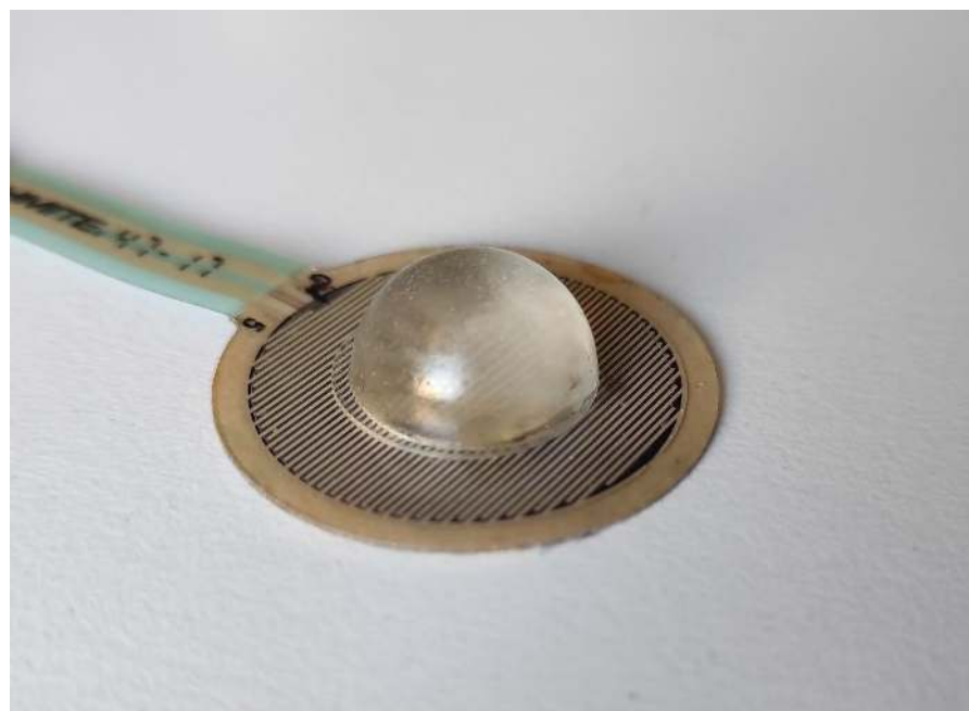
Figure 1. The FCG sensor used in the experimental tests.
