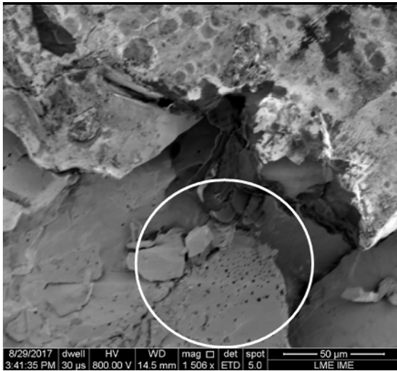
Figure 7. SEM image of sample A95, showing the porosity of alumina particles.
