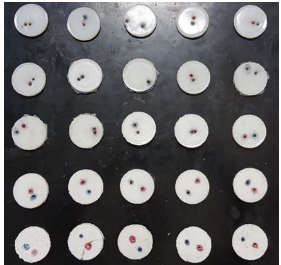
Figure 2. A00, A20, A40, A60 and A80 samples arranged in top-down rows, after the ballistic tests
