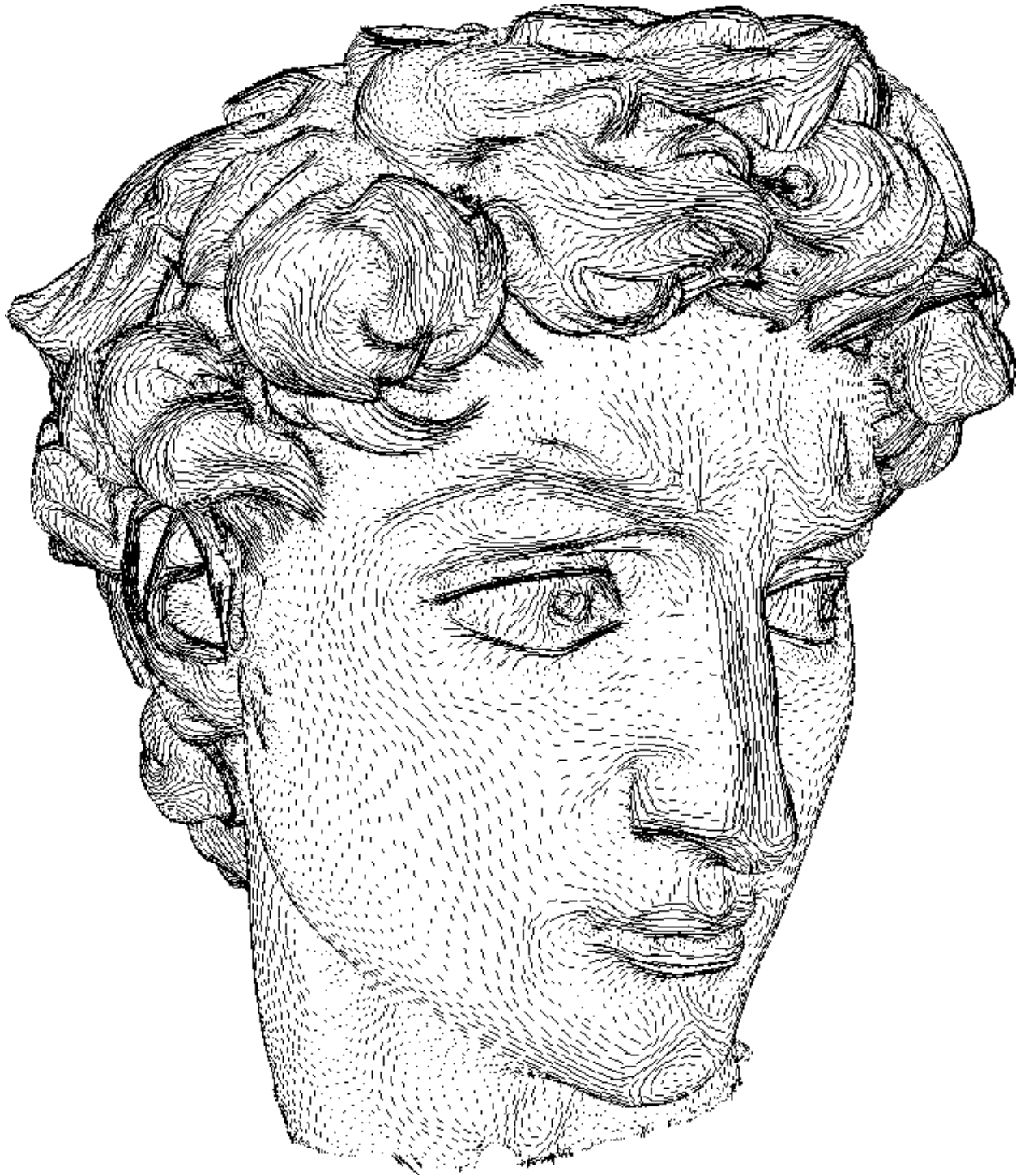
Figure 6: Directions of minimal curvature estimated on a mesh of Michelangelo's David. For each vertex, the averaging domain used for computations is the 2-ring of that vertex.
