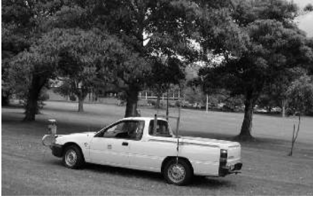
Figure 7: The vehicle used in our experiments is equipped with a 2D laser range finder and a differential GPS system. The vehicle’s ego-motion is measured by a linear variable differential transformer sensor for the steering, and a wheel-mounted velocity encoder. In the background, the Victoria Park test environment can be seen.
