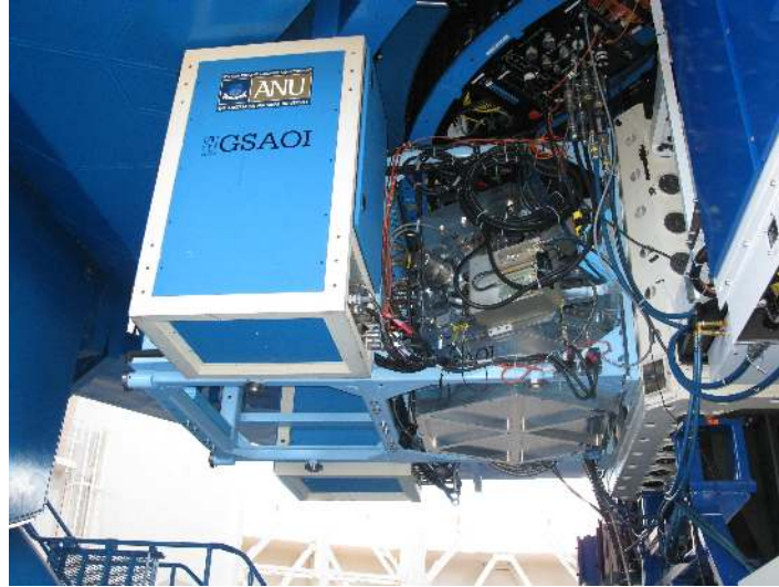
Figure 1. GSAOI after the installation on port 5 of the ISS. The Gemini South AO bench CANOPUS, is partially visible at the right corner of the picture.
