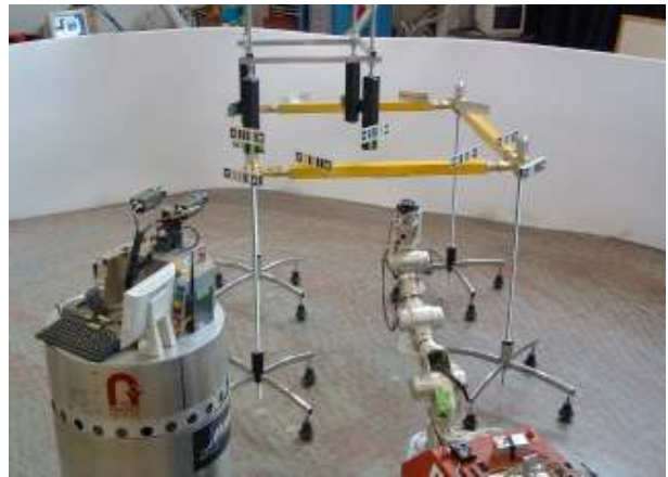
Fig. 1. Three robots with very different topology are used to autonomously assemble a square structure of four beams supported by four nodes.
