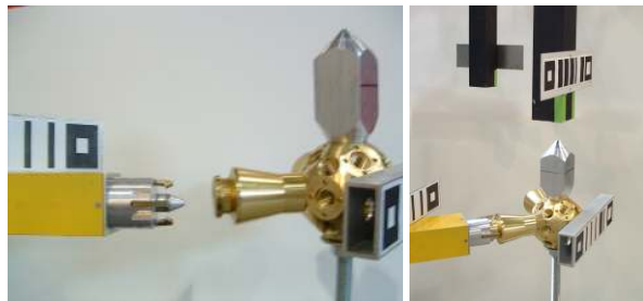
Fig. 3. Close-up of a beam being inserted into a node (left) and a node being braced by the crane (right).
