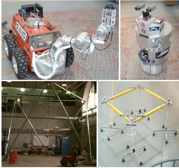
Fig. 2. The mobile manipulator (top left), the roving eye (top right), the RoboCrane (bottom left) and the completed structure (bottom right).
