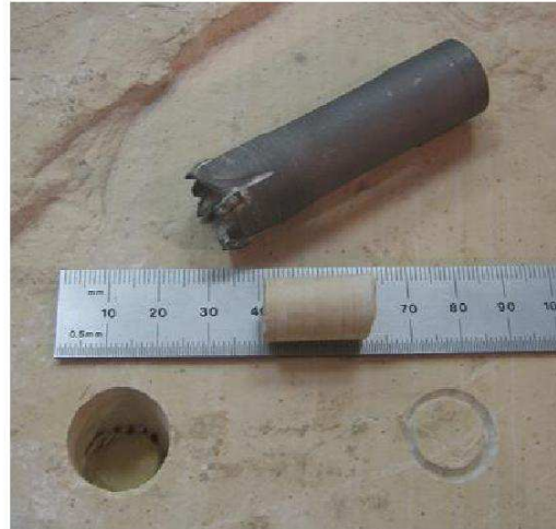
Figure 4: Core and bit from percussive coring test
