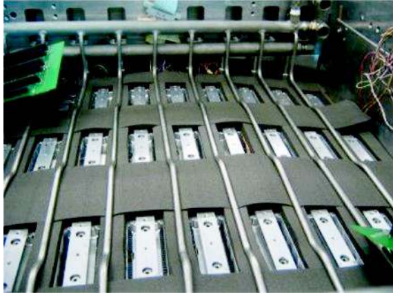
Figure 2: ECAL cooling scheme. On the left, the layer of insulating foam is shown on top of the grid. On the right, the cooling bars are shown with some of the cards inserted.
