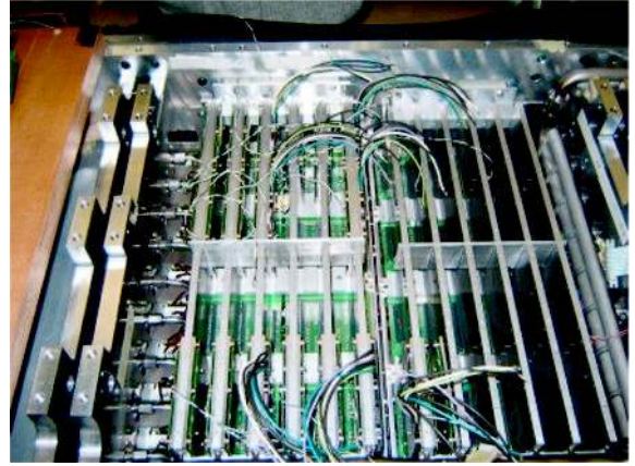
Figure 2: ECAL cooling scheme. On the left, the layer of insulating foam is shown on top of the grid. On the right, the cooling bars are shown with some of the cards inserted.
