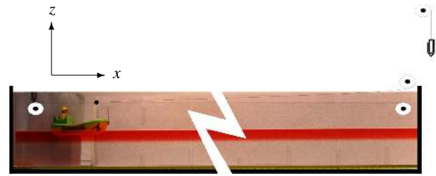
Fig. 2. Experimental setup of a boat dragged by a falling weight. The vertical force is converted horizontally through pulleys and an horizontal belt of fixed tension.
