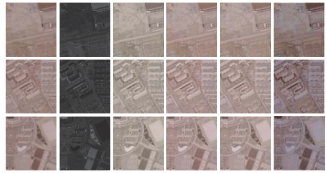
Figure 10: Qualitative results of Pan-Sharpening. From left to right: multi-spectral image, panchromatic image, and fused results of PCA, FISH, Brovey and our PMGI.
