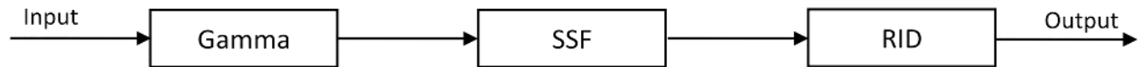
Fig 2. Flow chart of our proposed algorithm. A degraded image is enhanced through three steps in sequence: Gamma manipulation (Gamma), self-similarity filtering (SSF) and robust inverse diffusion (RID), respectively.
