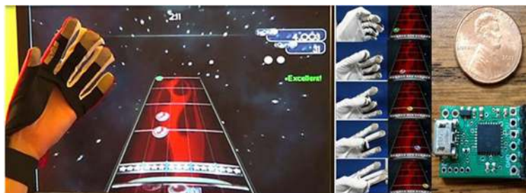
Figure 1 The MusicGlove is a sensorized glove that requires the user to make functional gripping movements to play a customized version of the open source music game called Frets on Fire , which was inspired by Guitar Hero . When the scrolling notes on the screen reach the white marker at the bottom, the user must make a specific grip associated with each note. The five grip types associated with each notes are shown (middle). When the electrical lead on the thumb touches one of the other five leads on the fingers, a custom-made controller (right) sends event data to a computer through an HID USB protocol.
