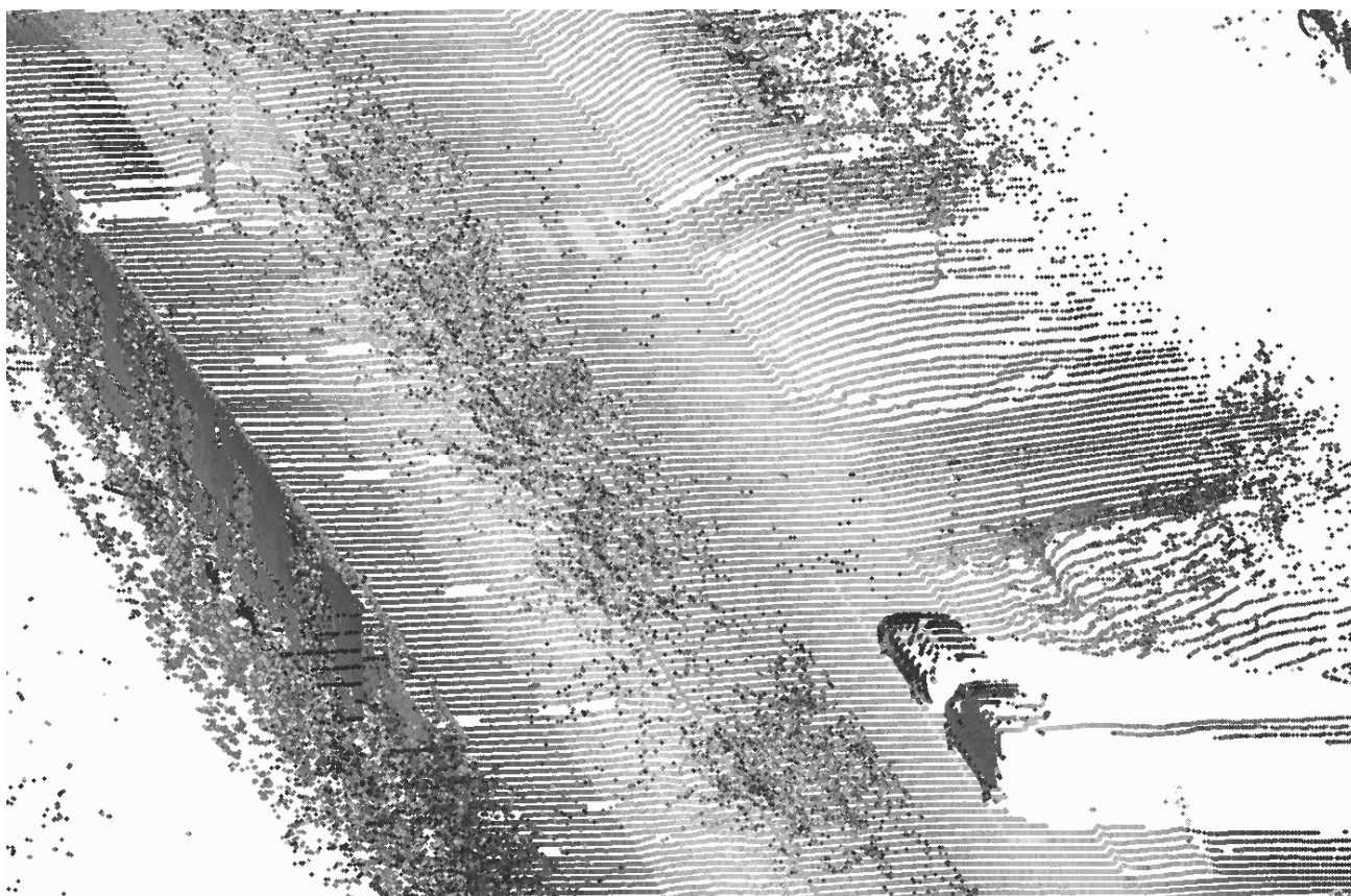
Figure 1. Part of the original point cloud showing a zebra crossing and a parking space line.
