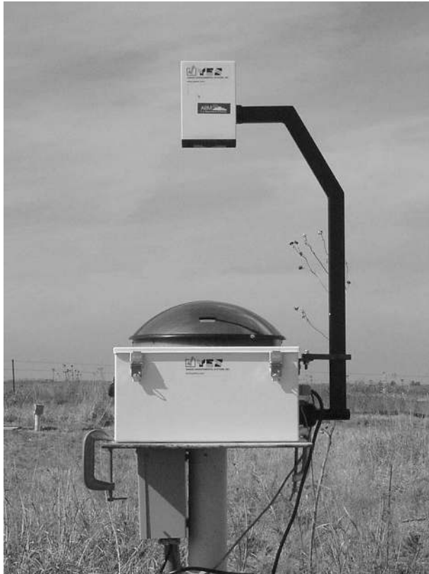
FIG. 1. YES TSI deployed at the ARM Climate Research Facility Southern Great Plains site in Oklahoma.
