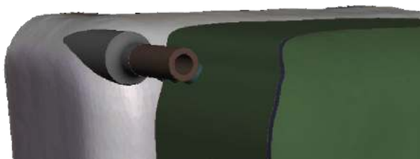
Figure 4: The mounting brackets allow the enclosure to easily be added to or removed from a legacy object.
