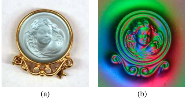
Figure 2. (a) This decorative pin consists of a glass bas-relief portrait mounted in a shiny gold setting. (b) The RGB image provided by the retrographic sensor. The pin is pressed into the elastomer skin, and colored lights illuminate it from three directions.
