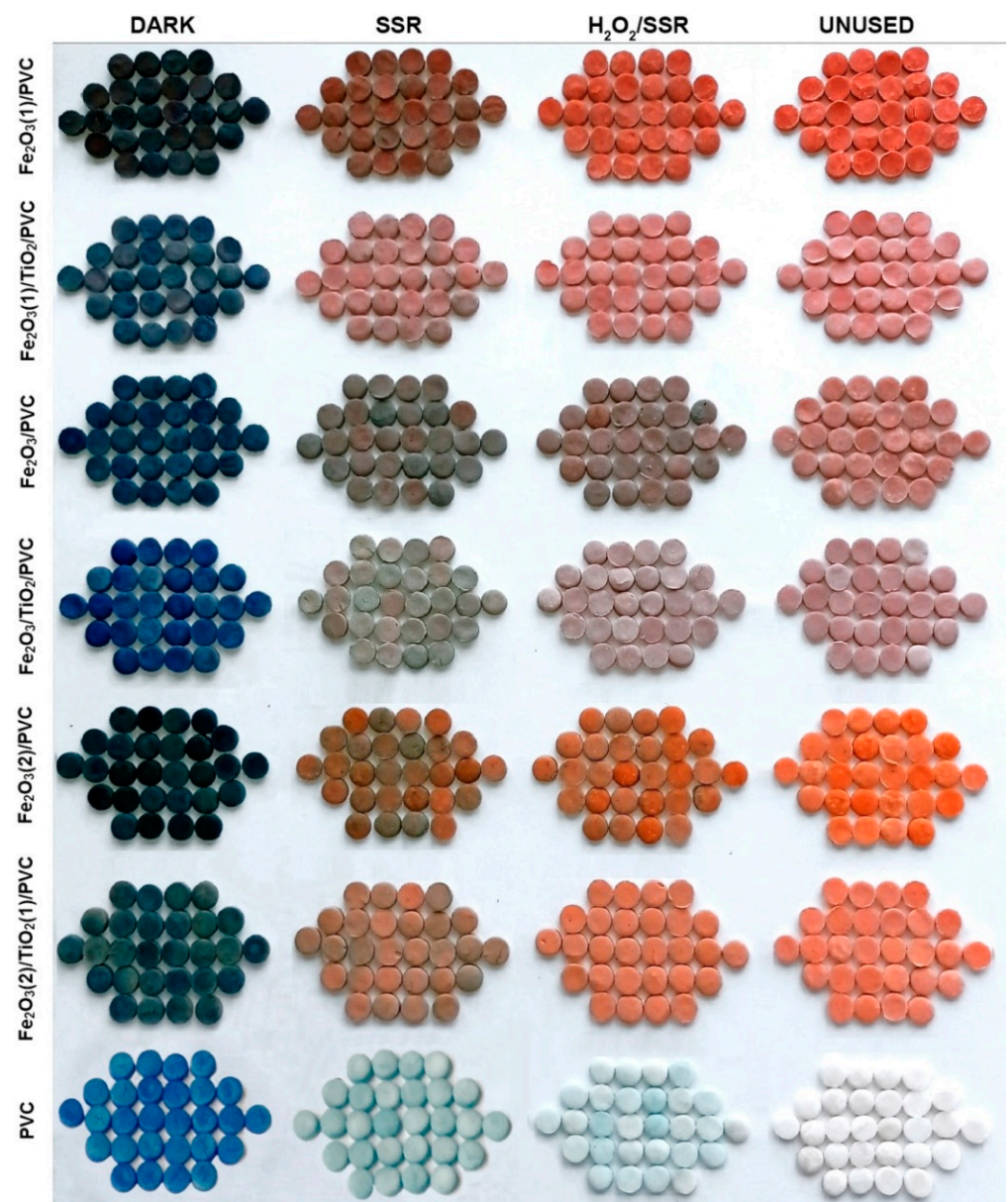
Figure 5. Photos of tablets after 180 min of the MB removal ( c_0 = 2.45 \cdot 10^{-2} mM) at a stirring rate of 490 rpm: first column (adsorption in the dark), second column (removal in the presence of SSR), third column (removal in the presence of SSR and \text{H}_2\text{O}_2 ) and fourth column (unused tablets).
