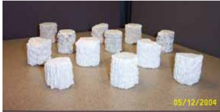
Figure 33: Wet/dry durability test samples after 12 cycles of being worked over with a Steel Brush
