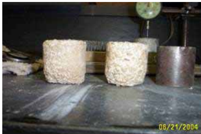
Figure 35: Comparison of specimens (left, center) after freeze/thaw tests with a steel cylinder (right) that is the same size as the specimens were initially
