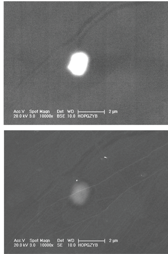
Fig. 5: SEM images of the same particle found in a ZYB sample taken in backscattering (top) and secondary electron (bottom) modes. Surface features are clearly visible in the SE image, while BS is mostly sensitive to chemical composition. The contrast around the particle in the SE mode is presumably due to a raised surface in this place.
