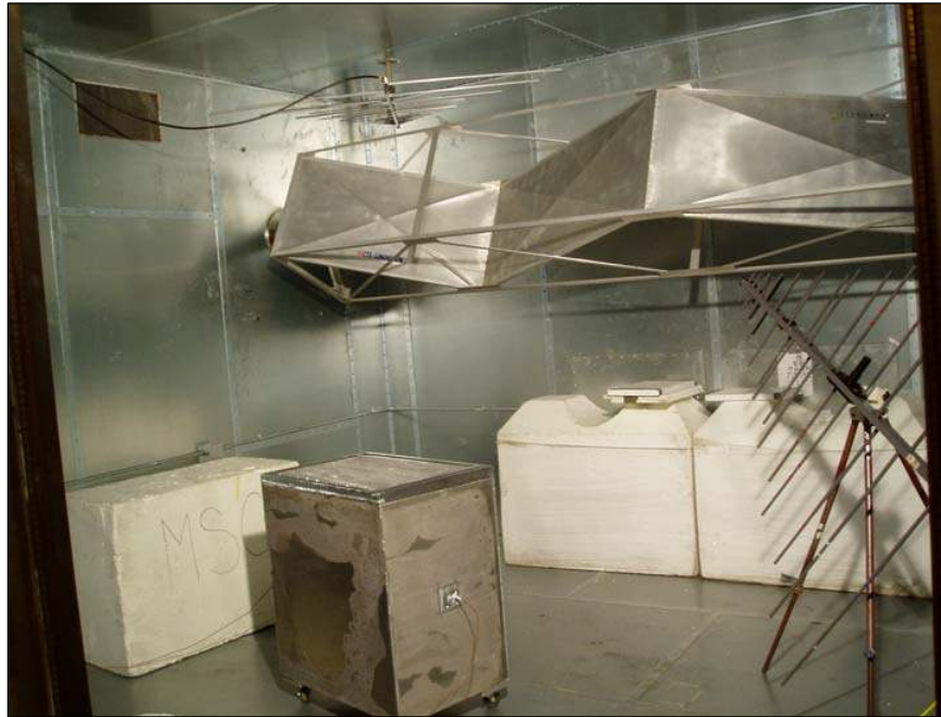
Figure 2-1. Typical Reverberation Chamber Setup
