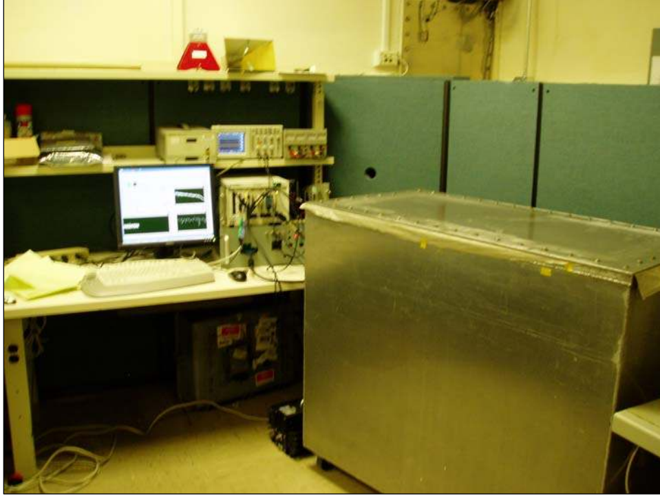
Figure 3–8. NSWCDD “Coffin” Chamber Fitted with Removable Top Plate
