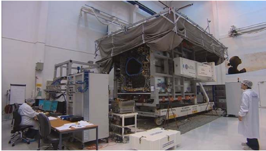
Fig. 13. Using the VIRC for the “sniff and spray test” for satellites. The “sniff and spray tests” are leakage tests on the several thousands of waveguide junctions in a high-tech communication satellite. This test takes normally four weeks with conventional test setups, reduced to few days when the VIRC is used.
