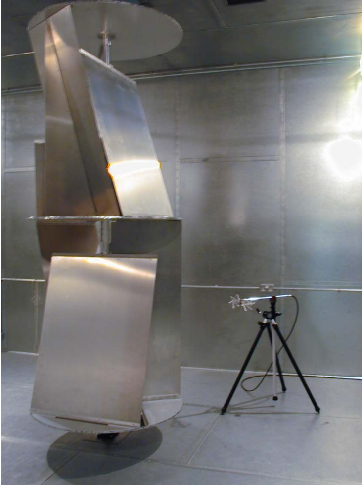
Fig. 9. Irregular reconfigurable stirrer in the RC at NPL, based on detachable aluminum stir blades and hinges that are attached to metal honeycomb disks using Velcro®. Photo extracted from [13].
