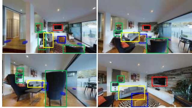
Figure 2. Object bounding boxes (BBox) in our simulator. The BBox size and aspect ratio of the same object may change after the agent moves to another viewpoint or changes its camera view.
