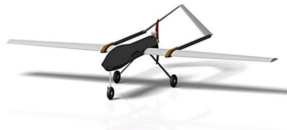
Fig. 1. Reconstruction of the fuselage in CATIA and the finalized 3D CAD of the JAVELIN UA.
