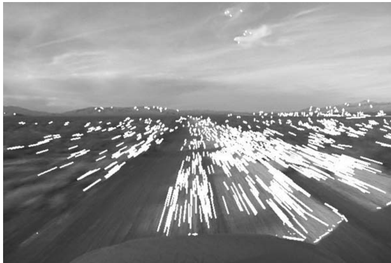
Figure 2. White lines represent the optical flow field in a typical desert driving scene (the length of flow vectors has been scaled by a factor of 2 for clarity).
