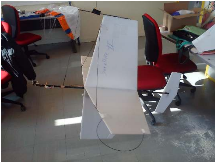
Fig. 11. The Satellite 2 prototype. The horizontal wing was used to generate the lift used to counter weight, and the vertical wing was used to produce a lift force for accelerating the kite.
