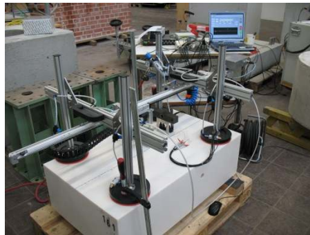
Figure 2. Half-automatic scanner for the ultrasonic measurements at polyamide and concrete
