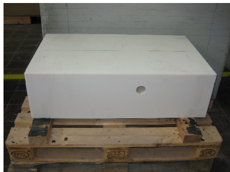
Figure 3. Polyamide specimen with hole drilled parallel to the surface
