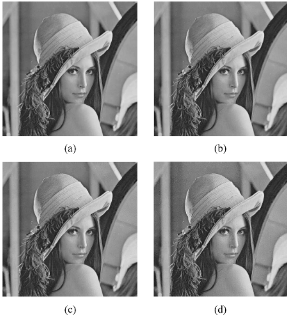
Fig. 5. Original and watermarked grayscale Lena images. (a) Original. (b) 44.87 dB with 0.30 bpp. (c) 37.82 dB with 0.65 bpp. (d) 32.92 dB with 1.00 bpp.
