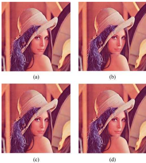
Fig. 8. Original and watermarked color Lena images. (a) Original. (b) 44.34 dB with 0.60 bpp. (c) 39.62 dB with 1.30 bpp. (d) 34.90 dB with 2.00 bpp.
