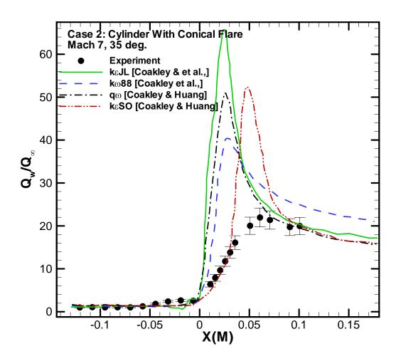
Fig. 12: Surface heat flux turbulence model comparisons (part 2) for Case 2: Cylinder with Conical Flare at 35 deg. (experiment by Kussoy and Horstman [34]).
