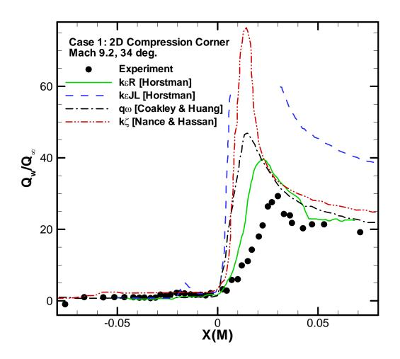
Fig. 7: Surface heat flux turbulence model comparisons (part 1) for Case 1: 2D Compression Corner at 34 deg. (experiment by Coleman and Stollery [33]).
