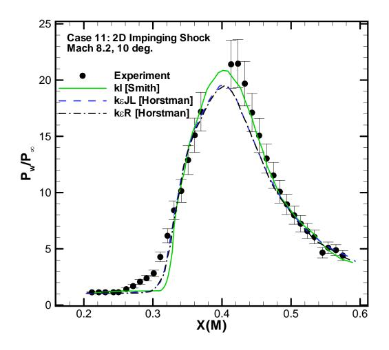
Fig. 17: Surface pressure turbulence model comparisons for Case 11: 2D Impinging Shock at 10 deg. (experiment by Kussoy and Horstman [40]).
