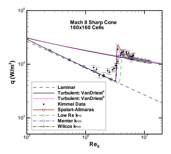
Fig. 3: Surface heat flux turbulence model comparisons for Case 10: Sharp Circular Cone (correlations are Van Driest<sup>a</sup> [74] and White's cone rule<sup>b</sup> [75] and experiment by Kimmel [119], [120]).
