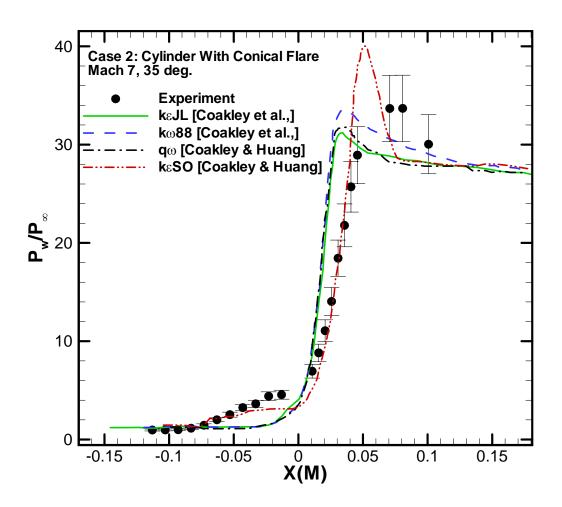
Fig. 10: Surface pressure turbulence model comparisons (part 2) for Case 2: Cylinder with Conical Flare at 35 deg. (experiment by Kussoy and Horstman [34]).
