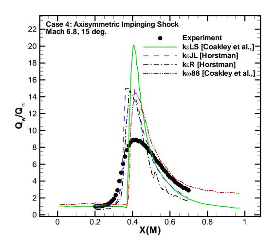
Fig. 16: Surface heat flux turbulence model comparisons for Case 4: Axisymmetric Impinging Shock at 15 deg. (experiment by Kussoy and Horstman [37], [164]).
