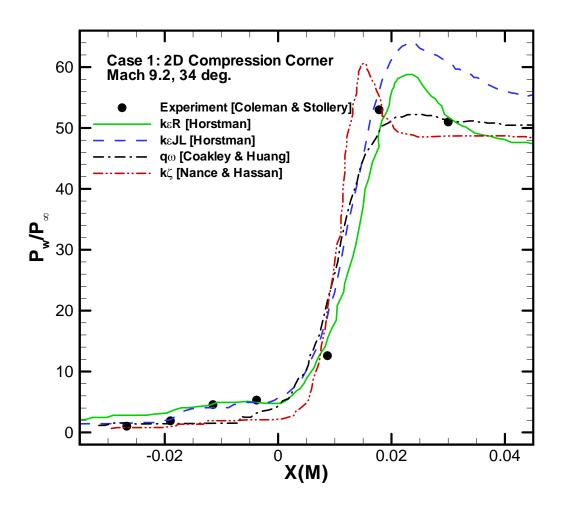
Fig. 5: Surface pressure turbulence model comparisons (part 1) for Case 1: 2D Compression Corner at 34 deg (experiment by Elfstrom [95]).
