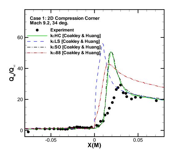
Fig. 8: Surface heat flux turbulence model comparisons (part 2) for Case 1: 2D Compression Corner at 34 deg. (experiment by Coleman and Stollery [33]).
