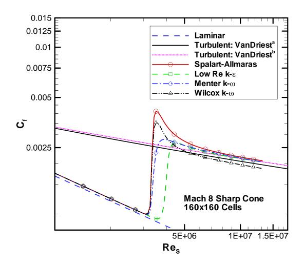
Fig. 2: Skin friction turbulence model comparisons for Case 10: Sharp Circular Cone (correlations are Van Driest<sup>a</sup> [74] and White's cone rule<sup>b</sup> [75]).
