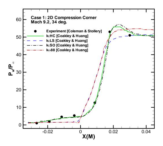
Fig. 6: Surface pressure turbulence model comparisons (part 2) for Case 1: 2D Compression Corner at 34 deg (experiment by Elfstrom [95]).
