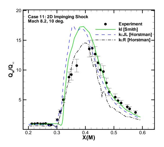
Fig. 18: Surface heat flux turbulence model comparisons for Case 11: 2D Impinging Shock at 10 deg. (experiment by Kussoy and Horstman [40]).
