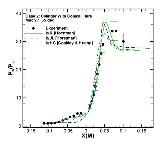
Fig. 9: Surface pressure turbulence model comparisons (part 1) for Case 2: Cylinder with Conical Flare at 35 deg. (experiment by Kussoy and Horstman [34]).
