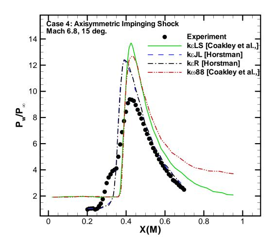
Fig. 15: Surface pressure turbulence model comparisons for Case 4: Axisymmetric Impinging Shock at 15 deg. (experiment by Kussoy and Horstman [37], [164]).
