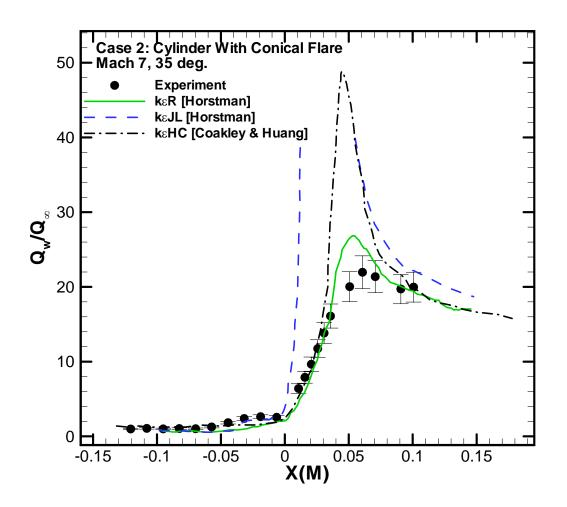
Fig. 11: Surface heat flux turbulence model comparisons (part 1) for Case 2: Cylinder with Conical Flare at 35 deg. (experiment by Kussoy and Horstman [34]).
