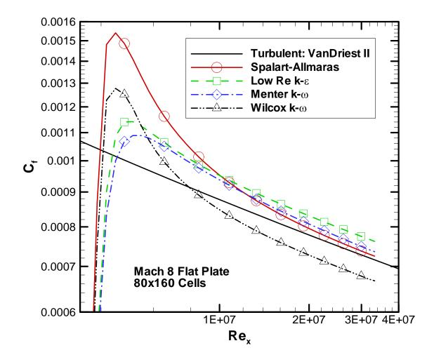
Fig. 1: Skin friction turbulence model comparisons (enlarged view) for Case 9: Flat Plate/ Cylinder (correlation is Van Driest II [115]).
