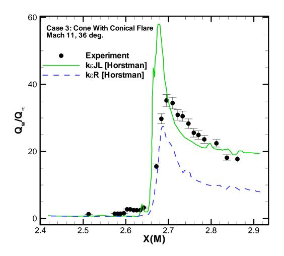
Fig. 14: Surface heat flux turbulence model comparisons for Case 3: Cone with Conical Flare at 36 deg. (experiment by Holden [44]).
