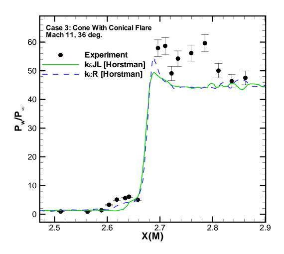
Fig. 13: Surface pressure turbulence model comparisons for Case 3: Cone with Conical Flare at 36 deg. (experiment by Holden [44]).
