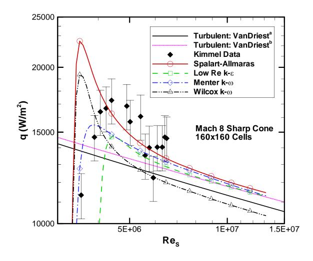
Fig. 4: Surface heat flux turbulence model comparisons (enlarged view) for Case 10: Sharp Circular Cone (correlations are Van Driest<sup>a</sup> [74] and White's cone rule<sup>b</sup> [75] and experiment by Kimmel [119], [120]).
