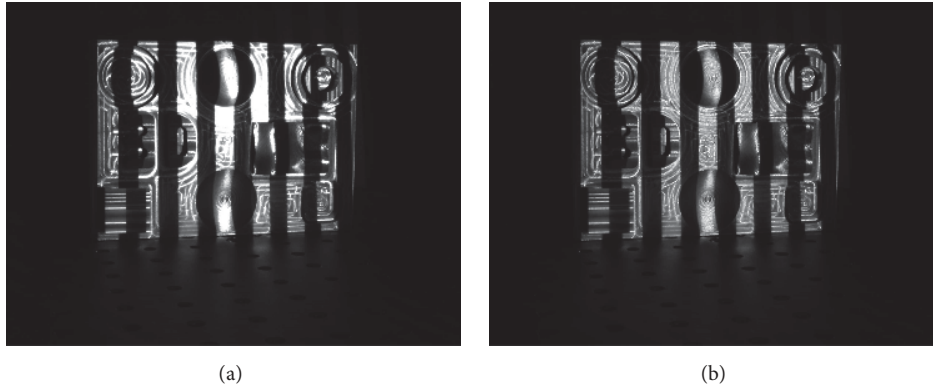
FIGURE 4: Comparison of results after using the technique proposed by Lin et al. [24]: (a) captured fringe image of an aluminum alloy workpiece with the conventional phase-shifting method and (b) captured fringe image of the same workpiece with the technique proposed by Lin et al. [24].
