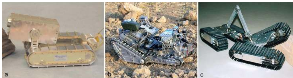
Figure 4. Tracked robots: Nanokhod (a, Klinker et al., 2007), Robhaz DT3 (b, Woosub et al., 2004) and Gunryu (c, Hirose et al., 1996).
