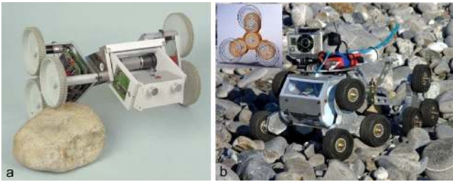
Figure 8. Stepping triple wheel hybrid robots: Spacecat (a, Siegwart et al., 1998); Epi.q (b, Quaglia et al., 2011).
