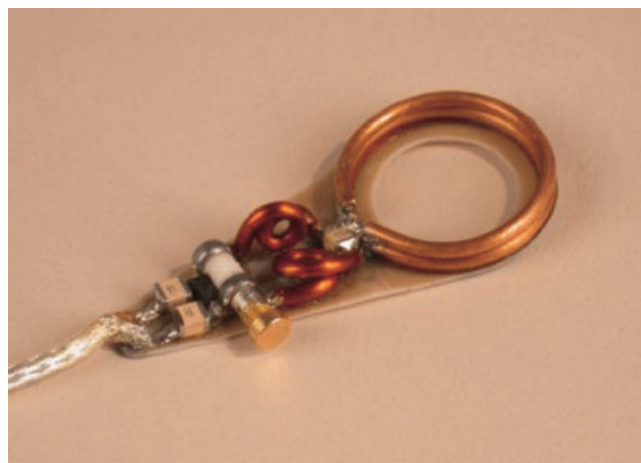
Figure 4. A 20 mm balanced surface coil with passive detuning. The diodes are hardly visible.
