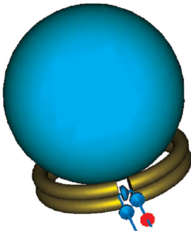
Figure 6. The surface coil and 'light load' simulation geometry, as described in the text. The lumped element capacitors are shown as small chamfered disks.
