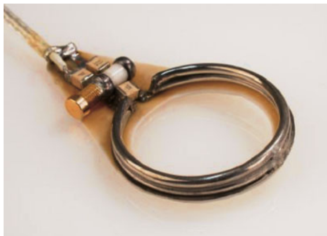
Figure 2. A 20 mm balanced T/R surface coil with heavy, magnetically compensated, parallel conductors. The thin acrylic coating over all the parts is not obvious, and the remote tune/match network, included in Fig. 1, is not shown here but is at the remote end of the feed cable.
