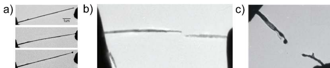
Figure 18: Electrical burn-out induced failure of the NEM switching element. a) Ball formation at the end of a Ge nanowire at the jump-in moment. Reprinted with permission from [10], copyright 2009 American Chemical Society. (b) GaN nanowire and (c) Mo 6 S 3 I 6 nanowire bundle break in the middle when the voltage is applied in the on state. Reprinted with permission from [96], copyright 2011 American Chemistry Society and from [8], copyright 2010 IOP Publishing.
