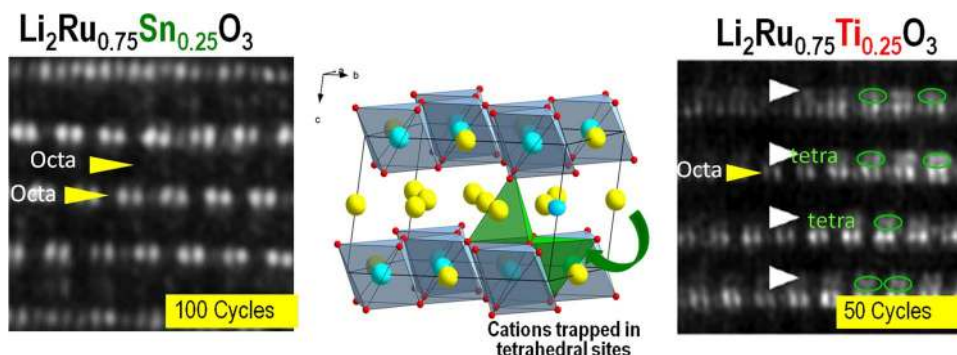
Figure 10. HAADF-SEM imaging of \text{Li}_2\text{Ru}_{0.75}\text{Sn}_{0.25}\text{O}_3 and \text{Li}_2\text{Ru}_{0.75}\text{Ti}_{0.25}\text{O}_3 electrodes recovered on the discharged state after 150 cycles and 50 cycles, respectively. The right image shows the presence of \text{Ti}^{4+} ions (white arrows) in tetrahedral positions as shown on the center structure. Such capturing on ions in tetrahedral sites was shown to increase upon cycling (from Ref. 120).
