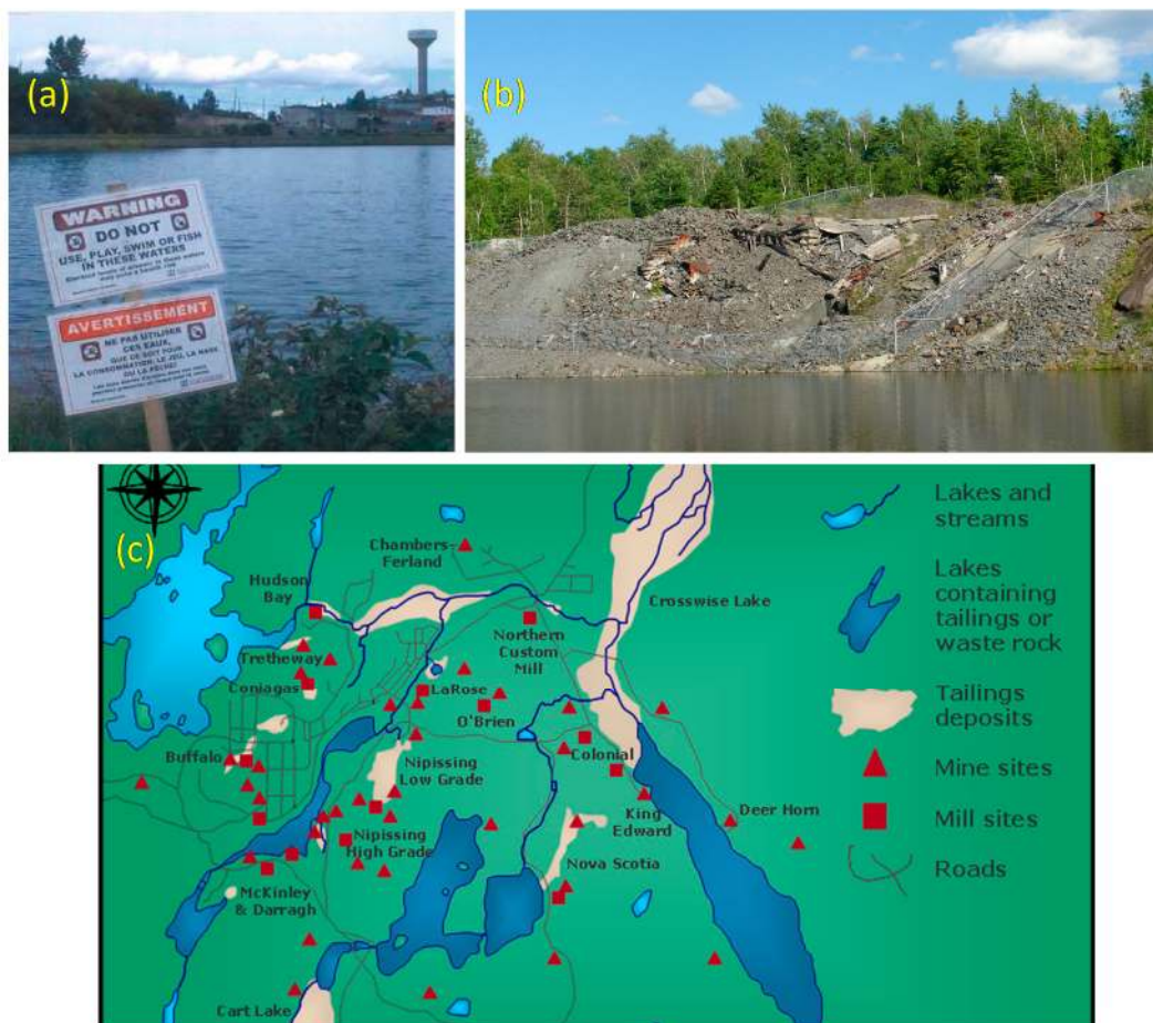
Figure 8. Water (a) and tailings (b) severely contaminated with arsenic; (c) Regional map of old workings in the region near Cobalt, Ontario, Canada with extensive tailings deposits indicated. Pictures from P.C. Miller, BacTech Environmental, reproduced with permission.
