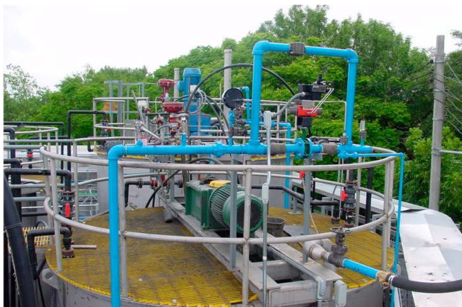
Figure 5. Biobleaching reactors at the Peñoles Mintek-Bactech demonstration plant at Monterrey, Mexico. Photograph by P.C. Miller, reproduced with permission.
