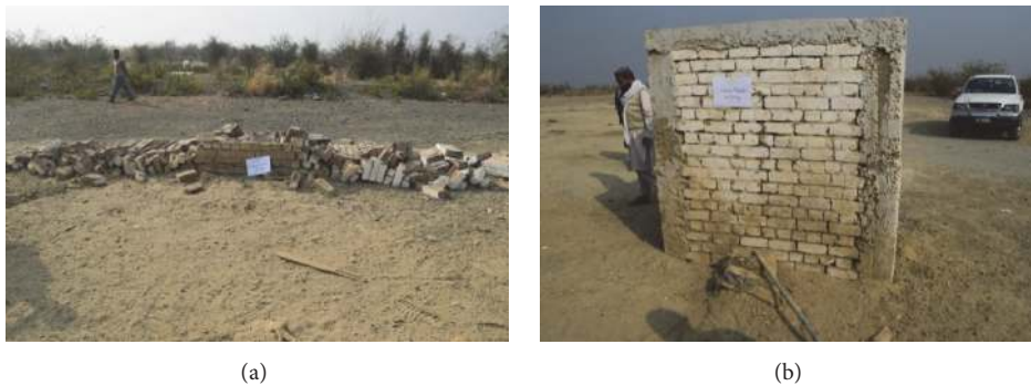
FIGURE 8: For scaled distance 1.89 \text{ m/kg}^{1/3} postblast scenario, (a) unreinforced masonry and (b) confined masonry.
