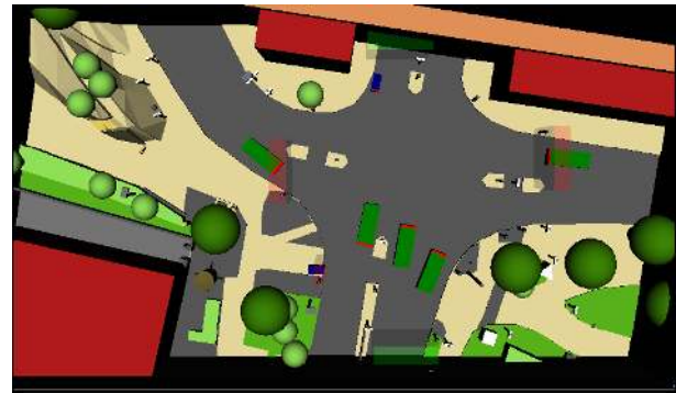
Fig. 7: The figure shows the haptic virtual model of Lund in Sweden [65]. Cars are realized by the green boxes while bicycles by blue boxes. Users could navigate using the PHANTOM and hear sounds of the environment; when hit, objects such as cars and bicycles also emitted an appropriate sound. Reproduced with permission.
