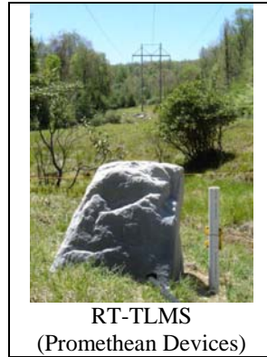
Figure 10. Commercial system based on electromagnetic field monitoring
