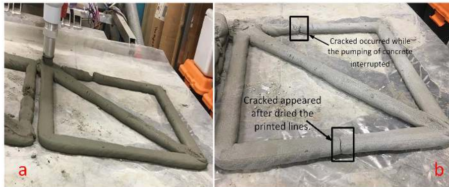
FIGURE 8 | (a) Printed mortar via extrusion printing, (b) Printed mortar by robot extrusion dried in the ambient temperature for 1 day.
