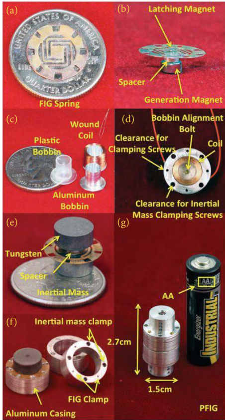
FIGURE 11: Fabrication of EM-VEH, reported by [40].
