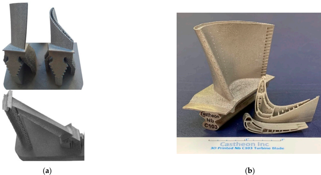
Figure 2. Metal and ceramic turbine blades produced via new manufacturing processes [13,14], and more in [15]. (a) Rotor Blades, (b) Airfoil with complex cooling features (courtesy: Castheon Inc.)
