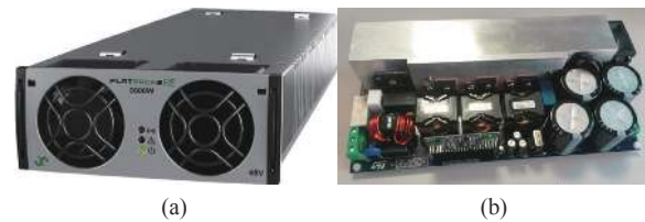
Fig. 1. Examples of hardware based on the conventional Boost PFC with Si SJ MOSFETs: (a) Eltek product AC/DC (PFC+LLC) product, 3 kW, 4.25 x 1.69 x 13 inch 3 [3]; (b) ST 3 kW PFC evaluation board, 9.6 x 4.3 x 1.4 inch 3 [4].
