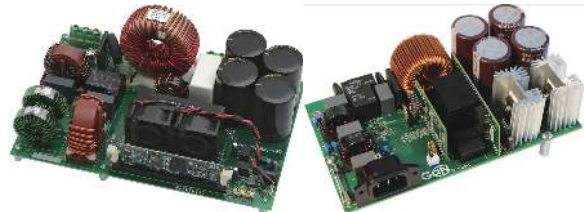
Fig. 8. Examples of hard-switching GaN totem-pole PFC: (a) Transphorm 4 kW, 66 kHz [29]; (b) GaN Systems 3 kW, 65 kHz [27].
