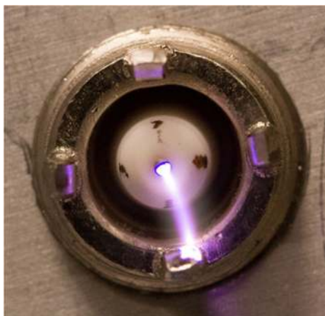
Fig. 8 Spark-like discharge device. Reprinted from [82] with permission
