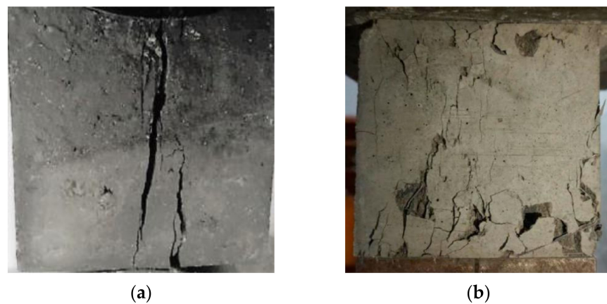
Figure 4. Compression failure of fiber-reinforced RAC: (a) [55]; (b) [67].
