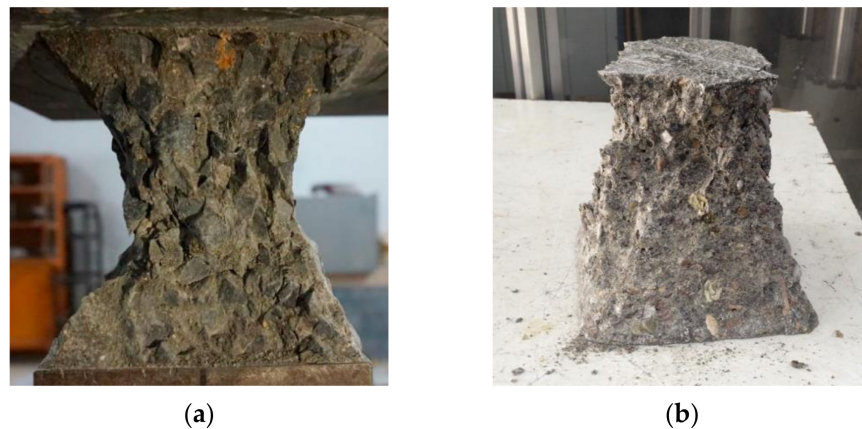
Figure 3. Compression failure of RAC without fibers: (a) [67]; (b) [68].
