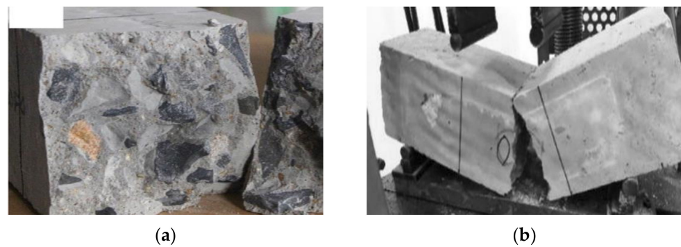
Figure 6. Flexural failure of concrete without fibers: (a) [88]; (b) [89].
