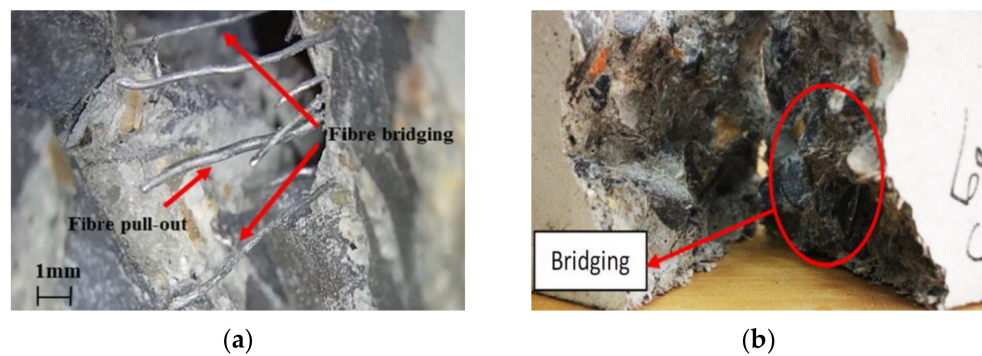
Figure 7. Flexural failure of fiber-reinforced concrete: (a) [70]; (b) [88].
