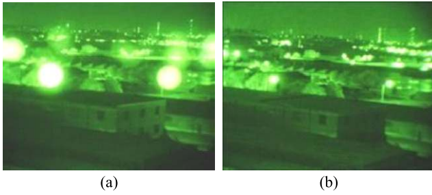
Fig. 16. Image generated by two night vision devices built using image intensifier tubes of different halo: (a) big halo, and (b) small halo (after Ref. 9).
