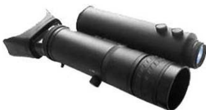
Fig. 37. Photo of an active night vision device type DM 740 from Dedal, Russia (after Ref. 71).
