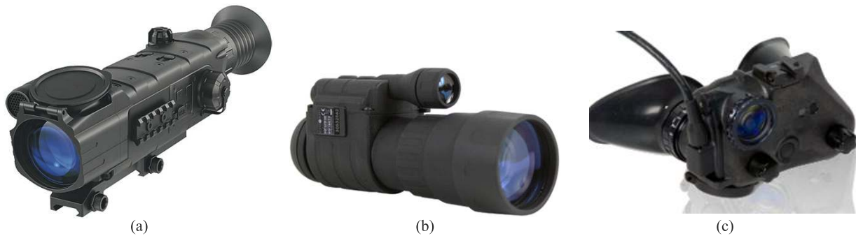
Fig. 28. Digital NVDs: (a) Pulsar Hindsight N550 digital sight, (b) Ghost Hunter 5×50 monocular (after Ref. 54), and (c) Monie-D goggles (after Ref. 55).
