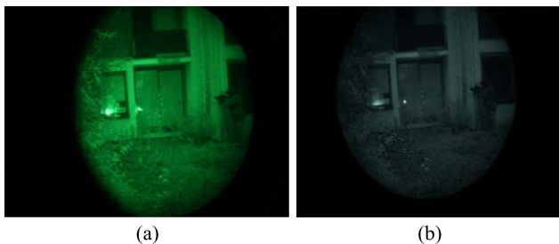
Fig. 21. Images of the same scene generated by two tubes with different phosphor: (a) typical XR5 tubes with P43 phosphor, and (b) Onyx tube with P45 phosphor (after Ref. 21).
