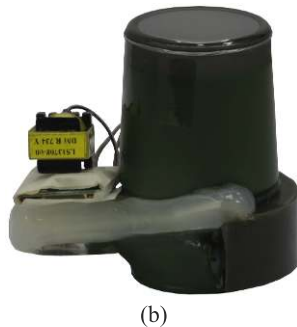
Fig. 10. Gen 1 tube: (a) diagram of a NVD built using a Gen1 tube, and (b) photo of Gen 1 tube with external electronic power supply.
