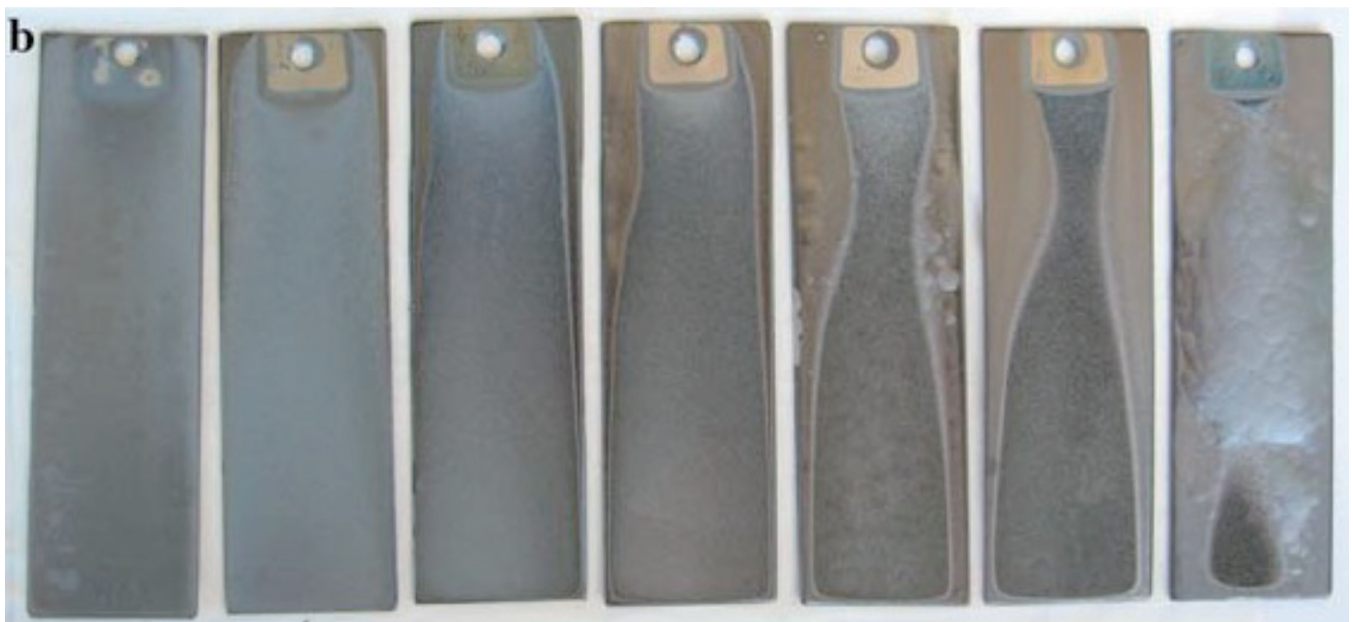
Fig. 17. Surface appearance of the samples oxidized at 1180°C 54) . Oxidation durations for the samples from left to right were 6,12,18,24,30,42,and 60 s, respectively.
