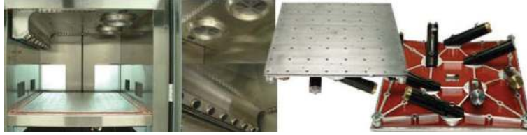
FIGURE 5: High accelerated life testing (HALT) chamber [15].
