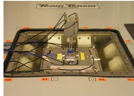
FIGURE 8: Simple structure under multiaxial loads [132].
