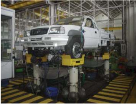
FIGURE 2: Four-post hydraulic simulator, from Awate et al. [17].
