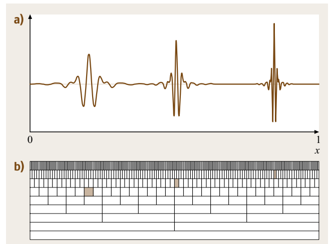
Fig. 22.29a,b Orthogonal quintic spline wavelets \psi_{j,i}(t) = 2^{j/2} \psi(2^j t - i) at different scales and positions: \psi_{5,6}(t) , \psi_{6,32}(t) , \psi_{7,108}(t) (a) and corresponding wavelet coefficients (b)
